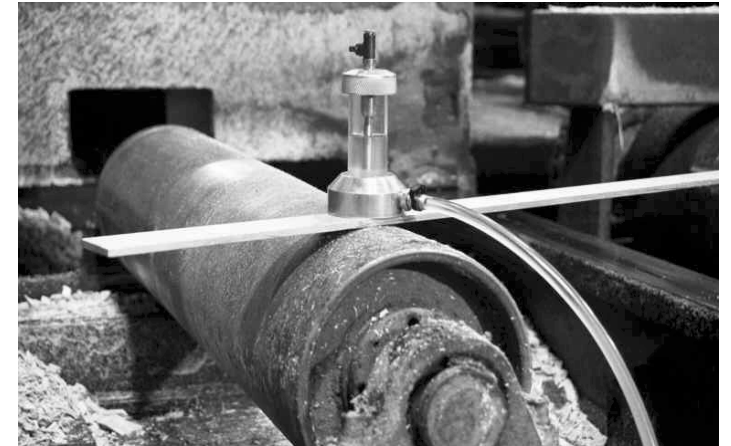
Hydro Level being used to check bed roll elevations
