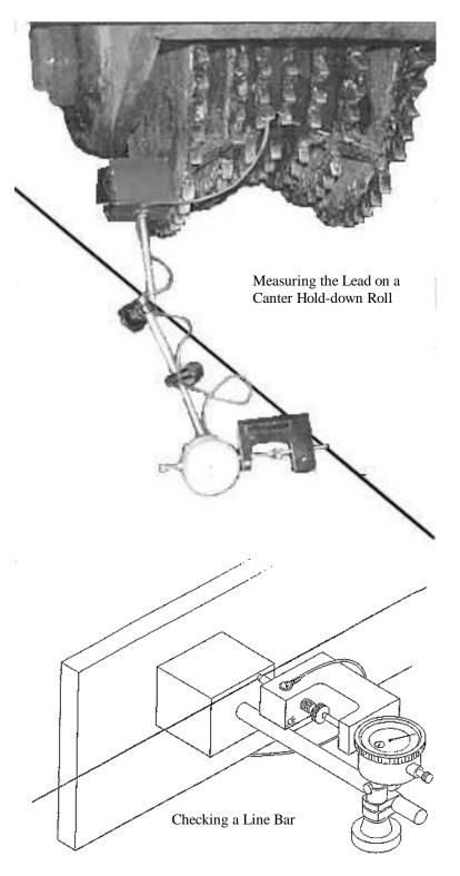
The Electronic Sensing Head was originally developed as part of the TKT Edger Alignment Kit for measuring if the arbour and rolls are 90 degrees to the alignment wire.
