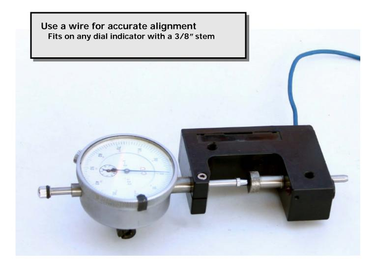
A small light comes on when the tip contacts the wire.
