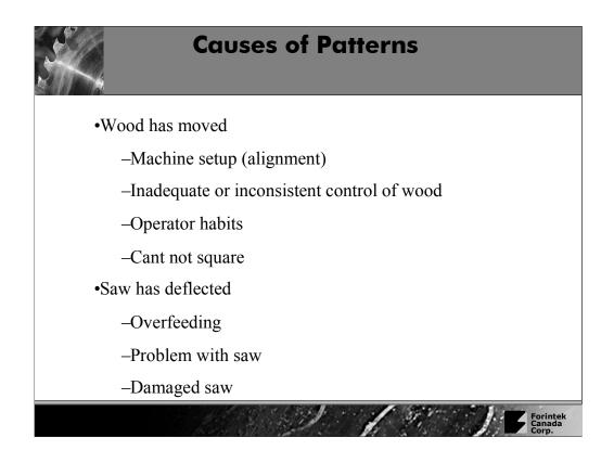
For example, a high within-board deviation points to saw deviation, it doesn't say why the saw deflected.
