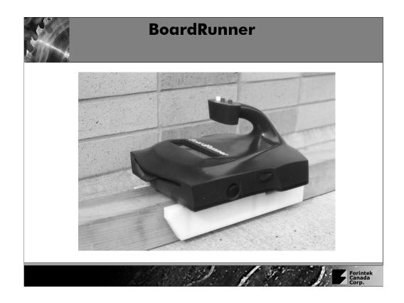
The BoardRunner runs on the edge of aboard taking thickness measurements as it is pushed along. Measurement spacing can be smaller than 1 inch, but typically as spacing of 2" or 3" is adequate.
