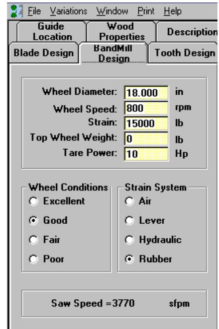
The screenshot shows the 'BandMill Design' section of the BandSel software. It includes input fields for 'Wheel Diameter' (18.000 in), 'Wheel Speed' (800 rpm), 'Strain' (15000 lb), 'Top Wheel Weight' (0 lb), and 'Tare Power' (10 Hp). Below these are radio button options for 'Wheel Conditions' (Excellent, Good, Fair, Poor) and 'Strain System' (Air, Lever, Hydraulic, Rubber). A 'Saw Speed' field shows '3770 sfp'. The interface also features tabs for 'Blade Design' and 'Tooth Design'.
